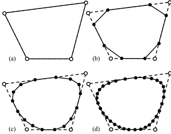
Fig. 1. Subdivision through Chaikin's corner cutting algorithm: (a) the initial control mesh; (b)-(d) control meshes after one, two and three subdivisions, respectively.
