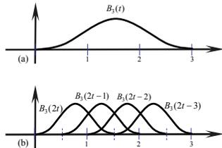
Fig. 4. Refinement of a 3<sup>rd</sup> order B-spline basis function through translation and dilation: (a) original basis function; and (b) translated and dilated copies of itself
