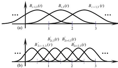
Fig. 5. Refinement of quadratic B-splines through mid-point knot insertion: (a) basis functions defined by a set of uniform knots; and (b) basis functions defined by refined knots through mid-point insertion
