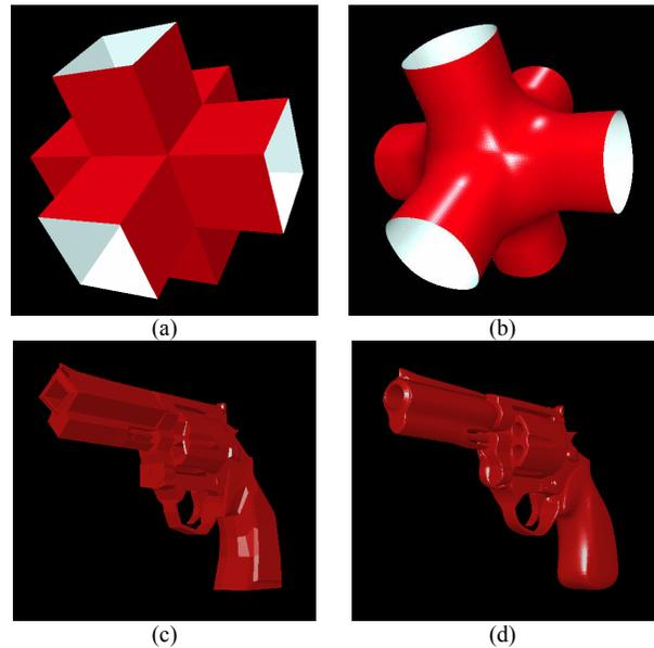
Fig. 11. Illustration of a pipe model (a)-(b) and a gun model (b)-(c) defined as a Doo-Sabin and Catmull-Clark surface, respectively. (a) and (c) initial control mesh, and (b) and (d) final limit surfaces.
