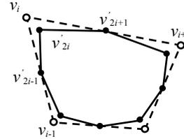
Fig. 6. Topological rules for cubic spline curve subdivision.
