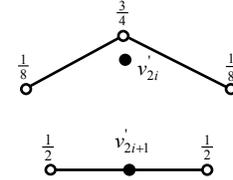
Fig. 7. Masks for cubic spline curve subdivision: (a) masks for updated corner vertices; and (b) mask for newly inserted edge vertex.
