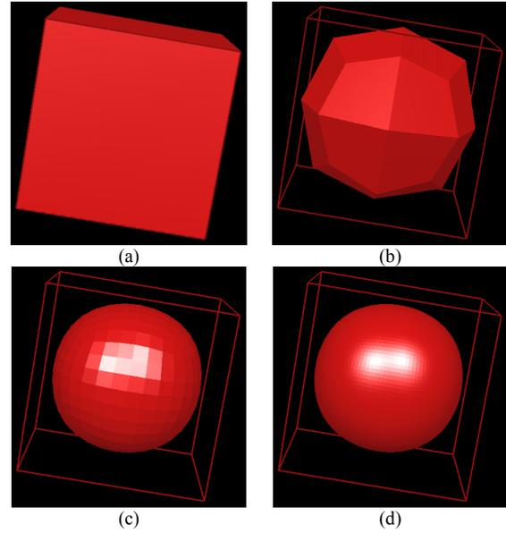
Fig. 10. Illustration of a Catmull-Clark subdivision surface: (a) the initial control mesh; (b) the control mesh after one level of refinement; (c) the control mesh after three refinement; and (d) the limit surface.
