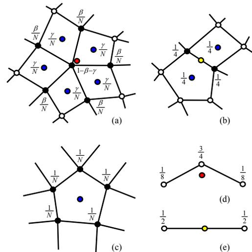
Fig. 9. General subdivision masks for Catmull-Clark surfaces: (a) mask for updated smooth V-vertices and darts; (b) mask for newly inserted E-vertices; and (c) mask for newly inserted face vertices.
