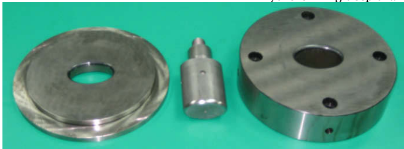
Holder Punch Die Fig. 3: The tools of elliptical cup drawing forming.
