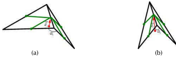
Fig. 4: The Laplacian vector \tilde{\delta}_i in the edge-based graph and the dihedral angle \alpha_i between adjacent faces in the primal domain. (a) The shorter \tilde{\delta}_i is, the larger \alpha_i will be. (b) The longer \tilde{\delta}_i is, the smaller \alpha_i will be.
