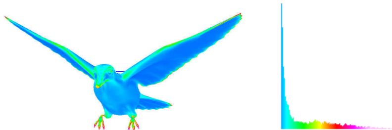
Fig.4: Left: visualize the principal curvature (maximum value) of each mesh vertex with color; Right: Corresponding histograms. Warm color represents global feature points, such as the claws, the wingtips and the back fringes of the wings. The front fringes of the wings are cool color, which are not global feature points, but they are very important to depict the shapes of the wings.
