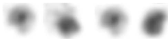
Fig. 2: From left to right, different scanned dots (600 dpi): A regular dot; an irregular dot; a mono-kernel dot; a multi-kernel dot.
