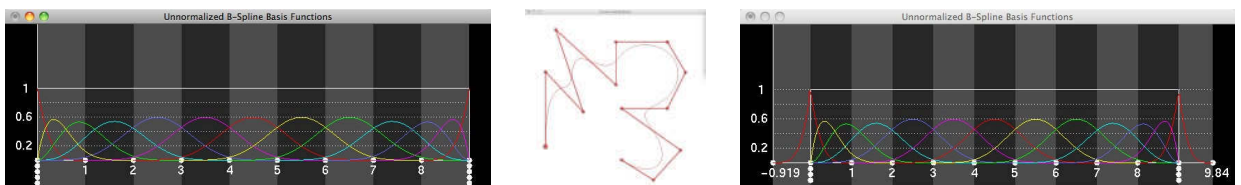
Fig. 8: The actual value of the first and last of the n+k+1 knots of a B-Spline do not affect the shape of the B-Spline curve: (a) blending functions for an order 5 clamped B-Spline, (b) the corresponding curve, (c) the blending functions after decreasing the first and increasing the last knot.
