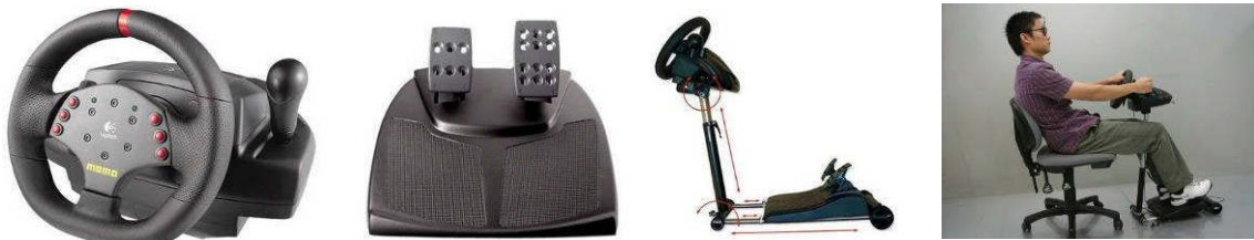
Fig. 4: MOMO Racing Force Feedback Wheel as driving panel for forklift truck simulation.
