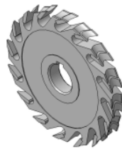
Fig. 5: Rendering of a CEFM cutter in CATIA V5 CAD software.
