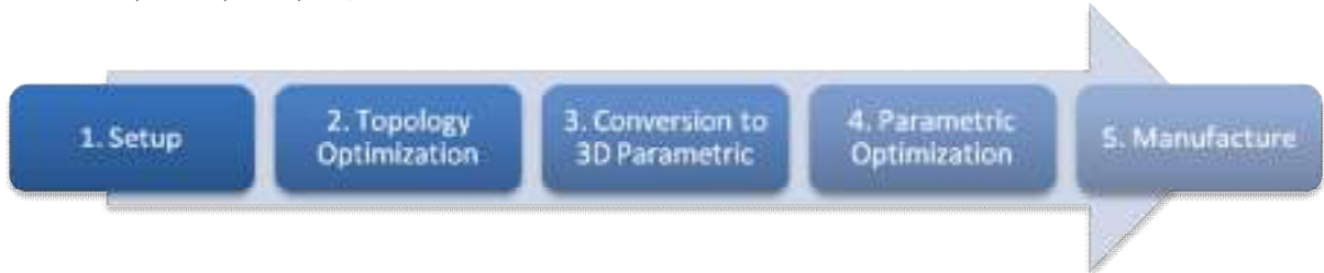
Fig. 1: Typical design process utilizing both TO and 3D parametric modeling.
