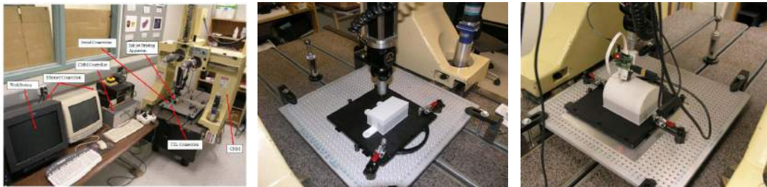
Fig. 1: CMM based 5-axis ink jet printing system architecture: (left) machine and sample part; (middle) touch trigger probe registration; (right) ink jet system mount.
