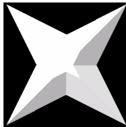
Fig. 1: A star-shaped parametric voxel element.
