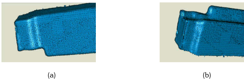
Fig. 10: Two zooms of the mobile phone point cloud (11 034 points) illustrating bad point sampling.
