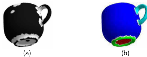
Fig. 7: (a) A “cup” model after thresholding and application of the morphological operators on the minimum curvature (the points above the threshold are shown with black color while points below the threshold are shown in white). (b) The segmentation of the cup is illustrated with colours denoting different regions (taken from [30]).
