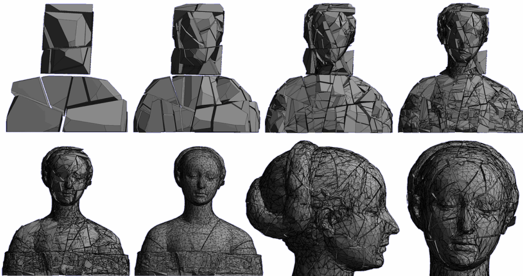
Fig. 7. Transformation from B-rep triangles to BSP: (a) progressive generation of model from triangles; (b) exploded view of the produced BSP; (c) a close view of the head.
