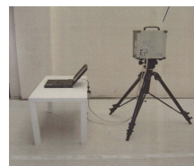
Fig. 3. Image of laser scanner on tripod.
