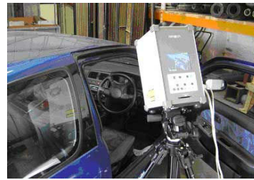
Fig. 4b. Interior scanning.
