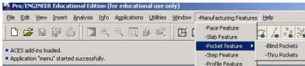
Fig. 12. Sub menus of manufacturing feature menu giving the set of manufacturing features in of expert machinist.
