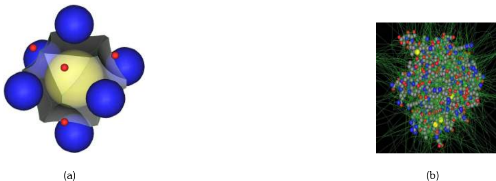
Fig. 4. Voronoi diagram of 3D spheres. (a) EVD for 15 spheres with 3 different types of radii, (b) EVD for spheres of Fig. 1
