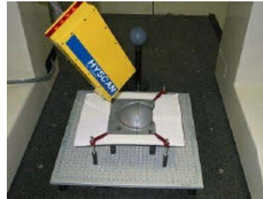
Fig. 6. Laser digitizer sheet metal grid measurement.
