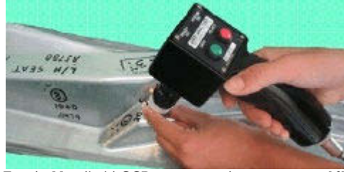
Fig. 4. Handheld CCD camera grid measurement [6].
