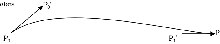
Fig. 8. Control parameters of the Hermite spline curve.
