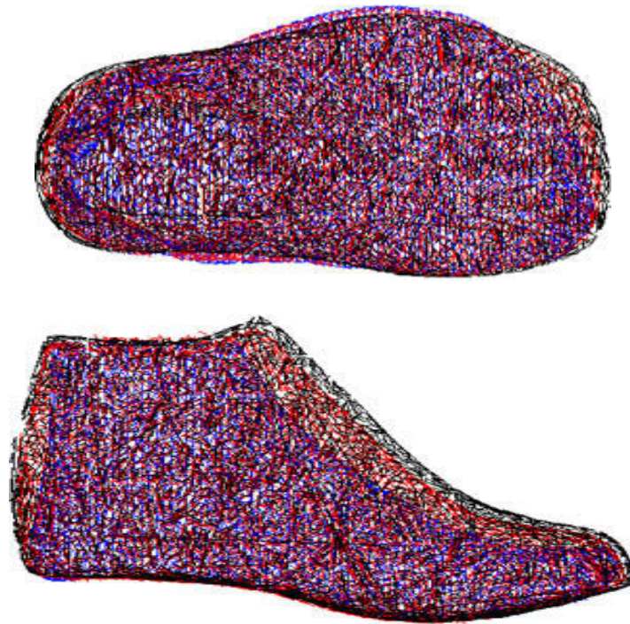
Fig. 7. The shape in red is the deformation result. The foot is shown in blue, and the original last form is shown in black.
