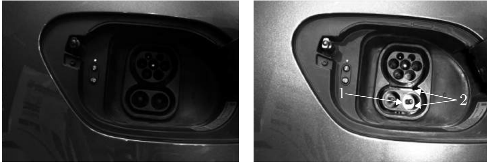
Figure 9: Examples of inlet camera images without and with LED light support.
