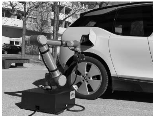
Figure 1: ACCS charging station prototype during outdoor tests.
