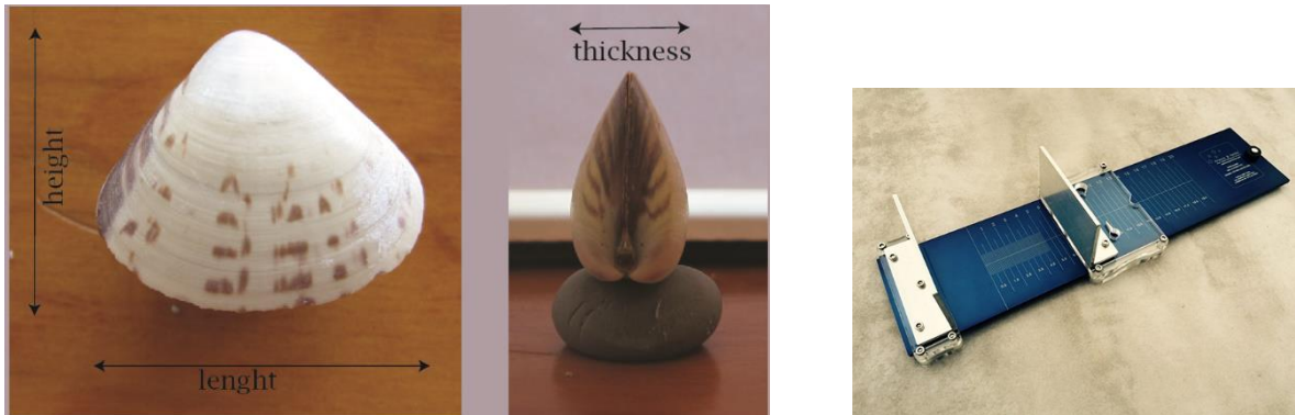
Figure 2: (a) Morphological measurements of a seashell and (b) Malachometer.
