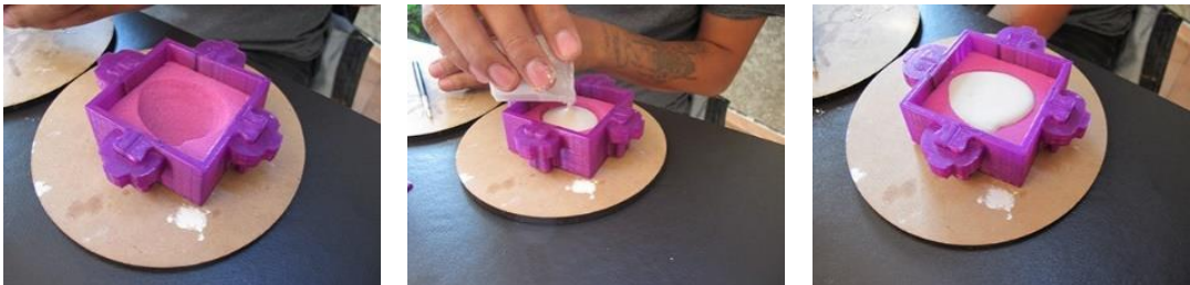
Figure 10: Mold and emptied of plaster.
