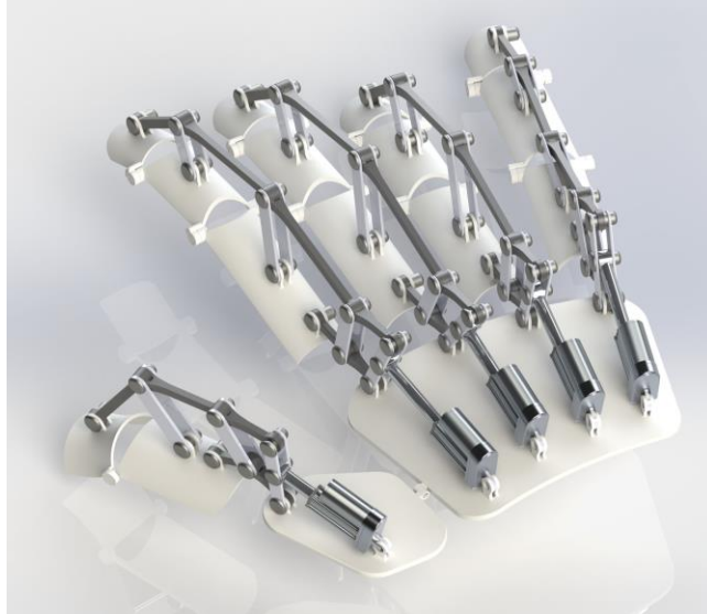
Figure 7: The hand rehabilitation device based on the proposed method using the square asymmetric correlation matrix.
