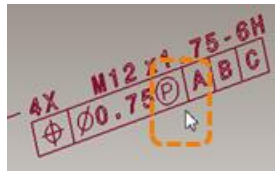
Figure 12: Missing project tolerance zone magnitude.
