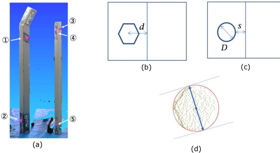
**Figure 13:** Experiment: (a) Steel Materials and Bolts, (b) Distance evaluated using Point-Cloud, (c) Manual Measurement using Vernier Calipers, and (d) Calculation of Bolt Position using the maximum Width.
