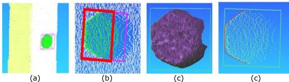
**Figure 7:** Process of hexagon fitting: (a) Cuboid for Bolt Points, (b) Points on the Scanner Side, and (c) Triangulation of Bolt Points, and (d) Boundary Points on the Scanner Side.
