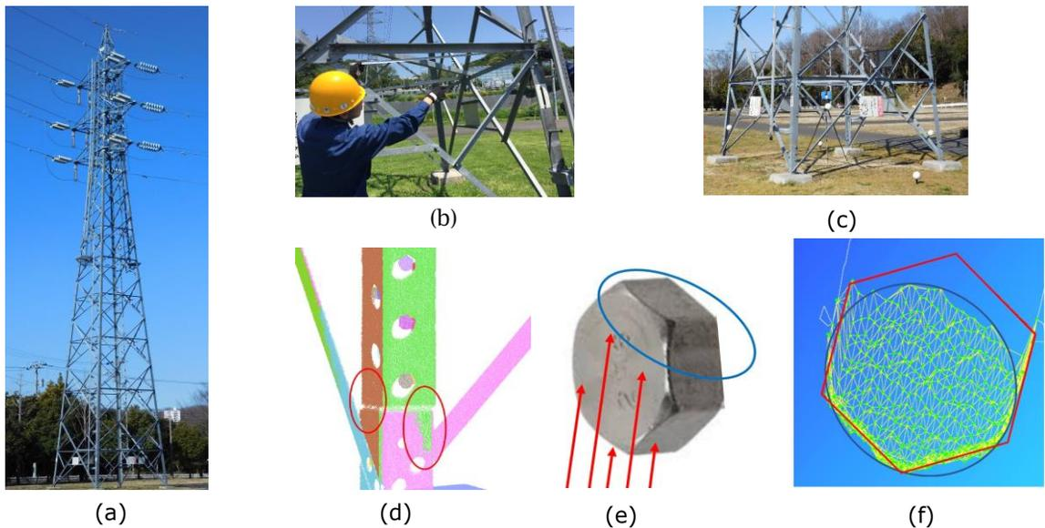
**Figure 1:** Power transmission pylon: (a) Steel Pylon, (b) Manual Measurement, (c) Laser Scanner on the Ground, (d) Detection of Planes, (e) Laser Scanning of Bolt, and (f) The Center Position of Bolt.
