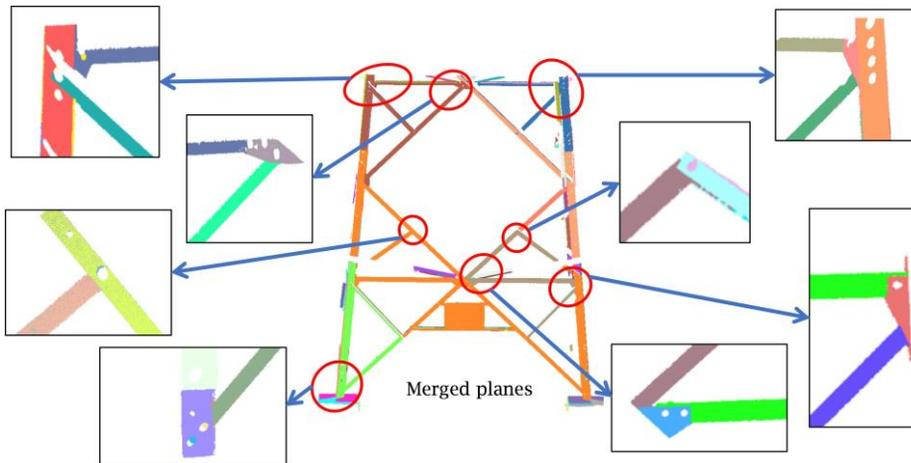
**Figure 9:** Segmented surfaces from merged planes.
