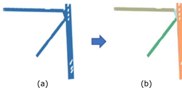
**Figure 5:** Segmented surfaces of steel materials: (a) Merged Plane, and (b) Detected Planes.
