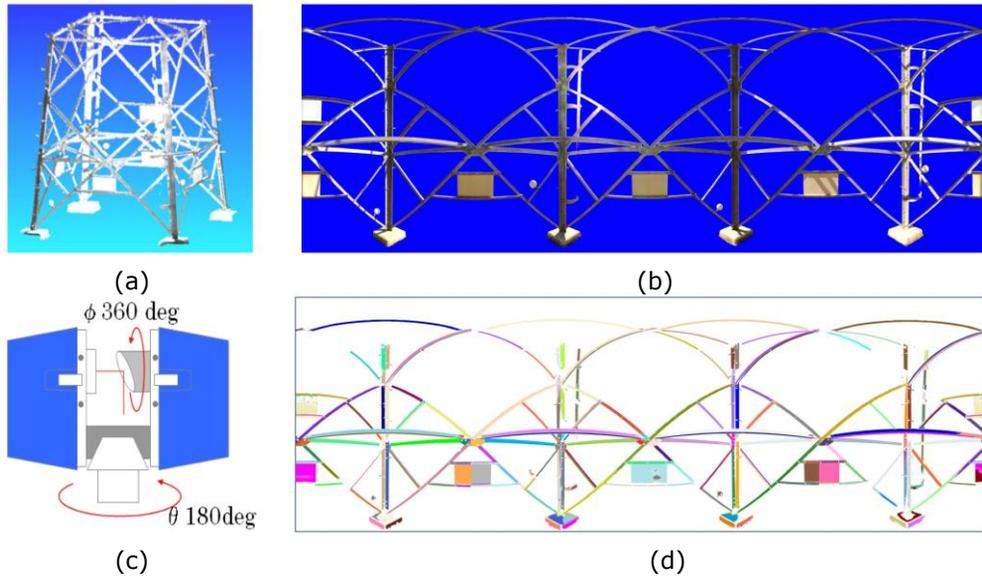
**Figure 2:** Plane detection using the RANSAC method: (a) Point-Cloud, (b) Direction of Laser Beam, (c) Mapping Points on the 2D Grid, (d) Detection of Planes on the 2D Grid
