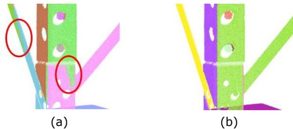
**Figure 3:** Merging adjacent planes: (a) Incorrectly Segmented Planes, and (b) Merged Planes.
