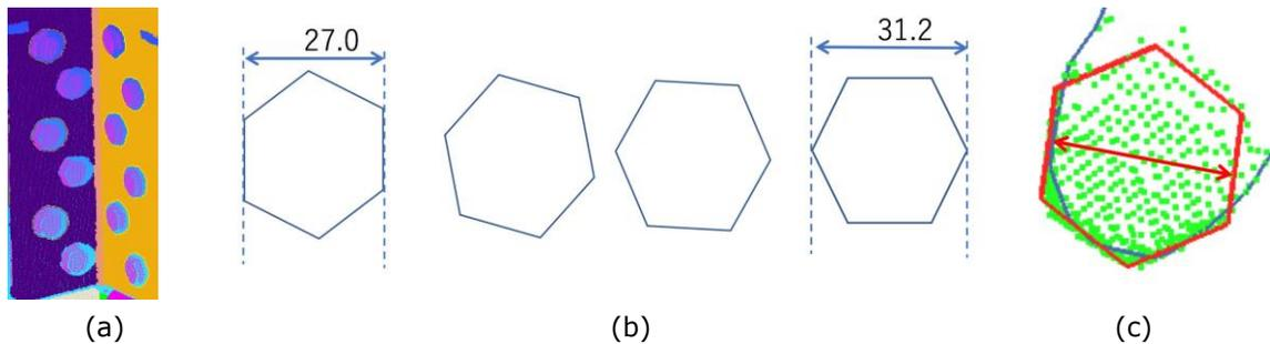
**Figure 6:** Bolt points: (a) Bolt Points, (b) Bolt Widths depending on rotation Angles, and (c) Calculation of Bolt Position by fitting a Hexagon.
