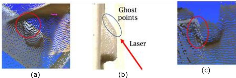
**Figure 12:** Failure cases in bolt detection: (a) Ghost Points of Bolt Head Surface, (b) The Reason why Ghost Points are generated, and (c) Bolt close to other Surface.
