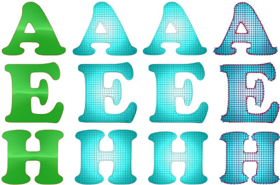
Figure 7: Three examples of converting the trimmed Letters A, E, and H into untrimmed T-splines. Left column: trimmed NURBS representation in Rhino; the second column: converted T-splines without optimization; the third and fourth columns: converted T-spline surfaces and T-meshes after optimization.
