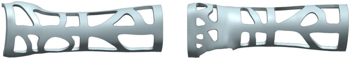
Figure 5: Final configuration of the reference pattern to be validated. The pattern is the result of manual modeling operations performed using the TO model as reference.
