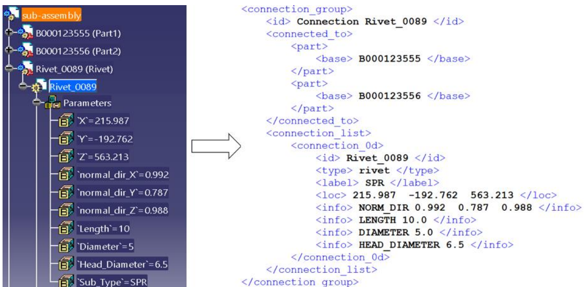
Figure 3: Comparison of native CAD joining technology data structure and xMCF joining technology data; exemplary displayed for a rivet connection.
