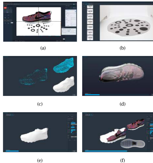
Figure 11: Operation workflow for 3D photo-modeling system: (a) object photo capturing software, (b) input mat photos and camera calibration, (c) model reconstruction, (d) camera alignment, (e) model optimization, and (f) texture mapping.
