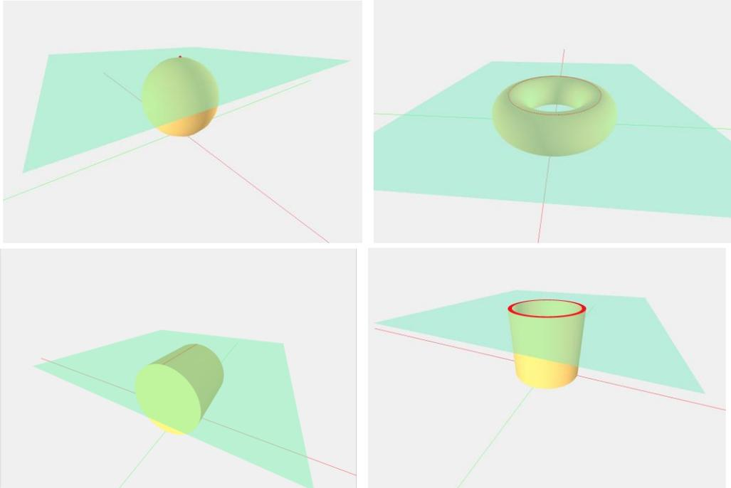
**Figure 1:** Point, curve, line and planar touch cases.
