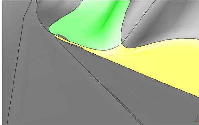
**Figure 6:** Overlapping surfaces in a complex NURBS model.
