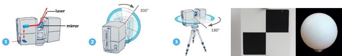
Figure 1: Faro 3D laser scanner: (a) The functionality of terrestrial laser scanners - FARO Focus3D X 330 Fig. (b). Checkerboard reference object and spherical object.
