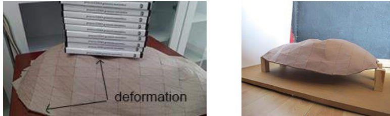
Figure 20: (a) First physical test and (b) Second physical test where the cardboard model after removing the weight is observed.
