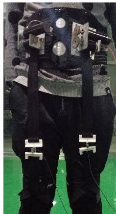
Figure 1: Walking assistive robotic suit.
