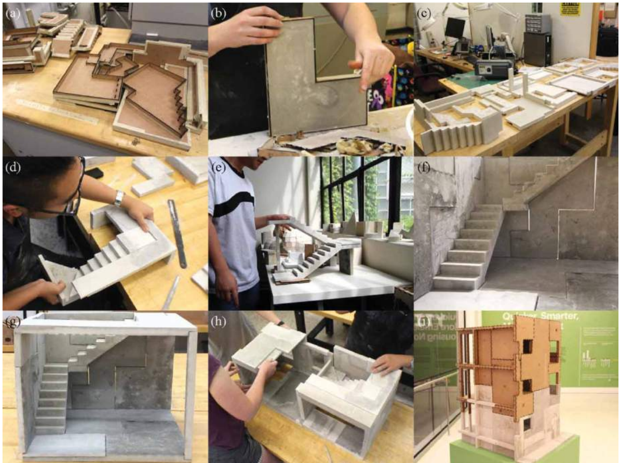
Figure 16. The process of making a modular house.
