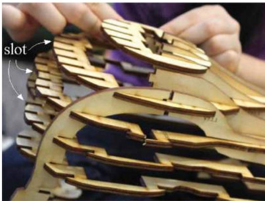
Figure 6. Tolerance affects the ease of assembly.
