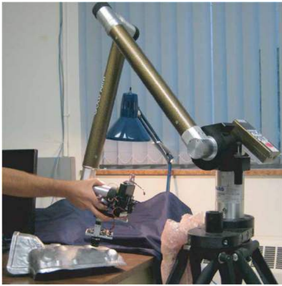
Figure 5. A hand-guided camera mounted on an articulated arm coordinate measuring machine (from [13], used with permission).
