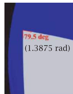
(c) Included angle between rake and clearance faces
