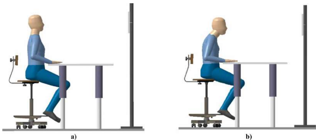
Figure 11. Comparison of the postures predicted with Safework (a) and with the proposed method (b) for a given working environment: \theta = 0^\circ , a = 230 mm b = 250 mm.
