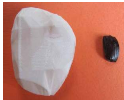
Figure 10. Comparison of 3D prototype with the elytra shape.
