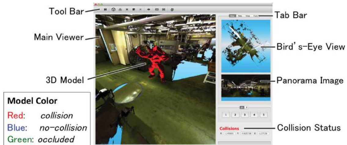
Figure 4. Collision detection system.
