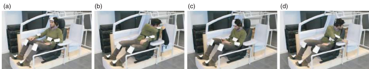
Figure 3. User during the execution of the four actions in the testing session: (a) researching of maximal comfort, (b) positioning of personal objects, (c) using of smart devices, (d) interacting with the back seats.
