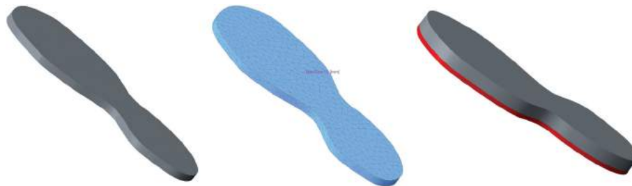
Figure 2. Models of the sole (from left to right): (a) 3D model of a single-layer sole, (b) the finite element mesh of the same sole, (c) 3D model of a double-layer sole.
