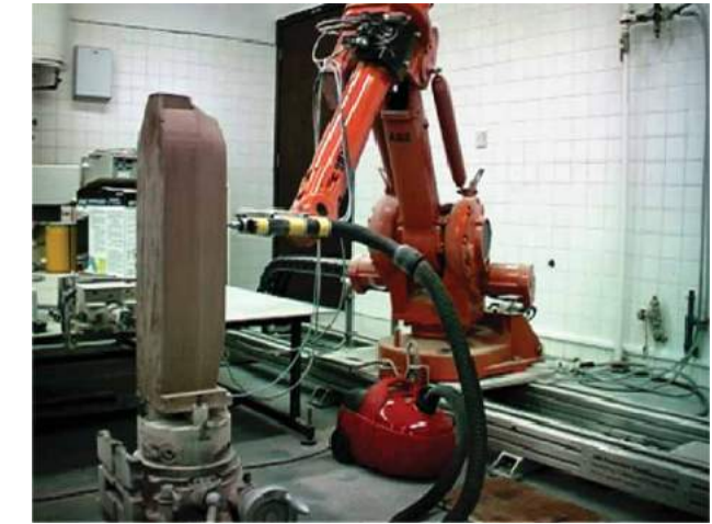
Figure 12. Actual machining process for a large ship model.
