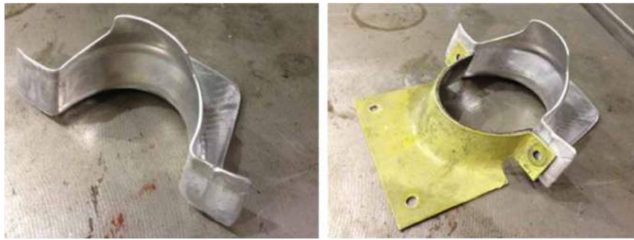
Figure 24. Successfully formed part (left) with the matching half in yellow color (right).
