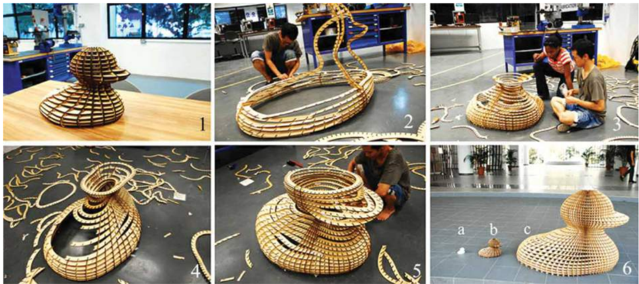
Figure 12. (1) Middle-scale model built of 20 horizontal layers. Large-scale model: (2–3) start of assembly and base parts, (4) oscillation of in-plane slots on horizontal layers, (5) assembly of the last 30 layers, and (6) comparison in size between (a) the original model used for scanning, (b) middle-scale, and (c) large-scale models build from the same starting scan.
