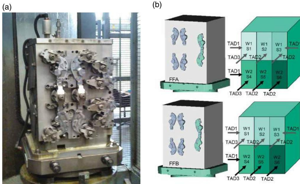
**Figure 5.** Pallet used for the industrial application (a) and two of the setups obtained from the pallet design system (b) where  $TAD_i$  = tool access direction for workpiece of type  $i$ ,  $W_i$  = workpiece of type  $i$ ,  $S_i$  = setup.
