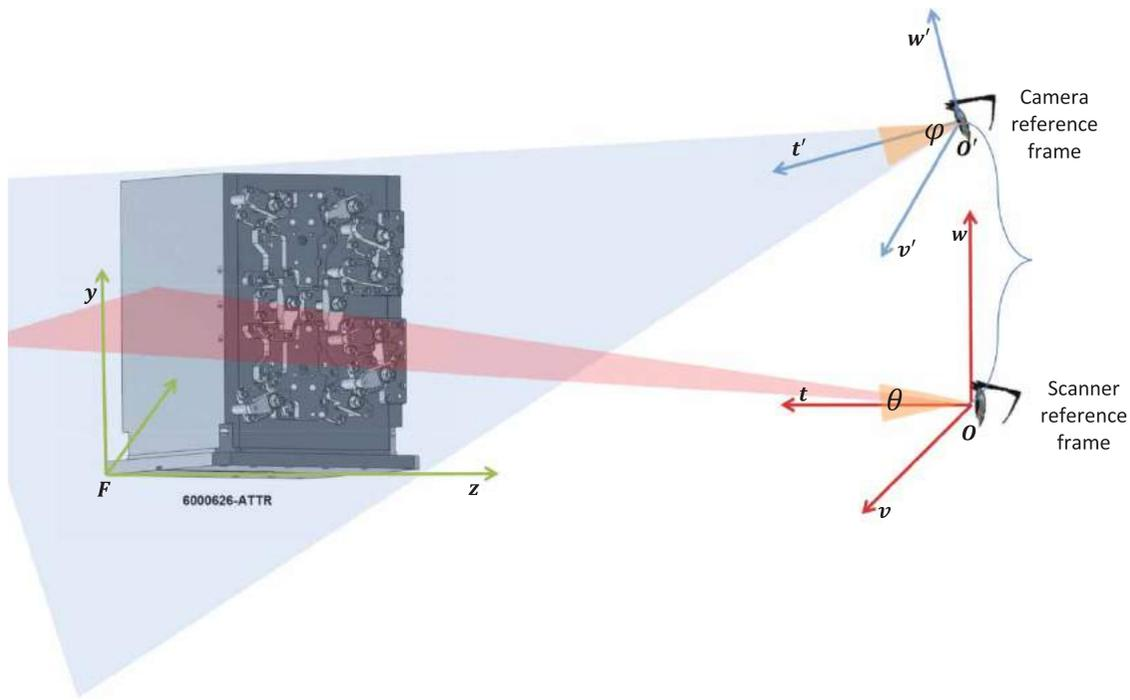
**Figure 4.** Simulated Pallet scan process.
