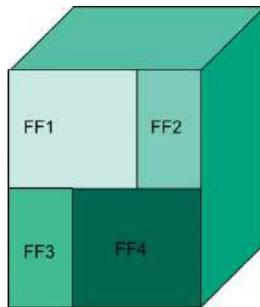
**Figure 3.** Example of a pallet fixturing faces (FFs).
