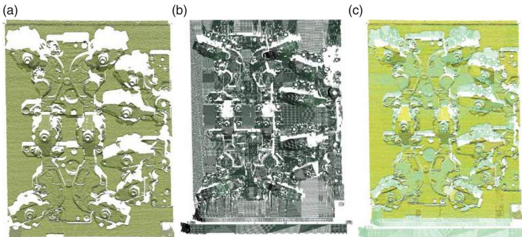
**Figure 6.** Acquired pallet point set (a), point set resulting from the visible point computation on the CAD configured pallet representation (b), overlapping of the above two point sets (c).
