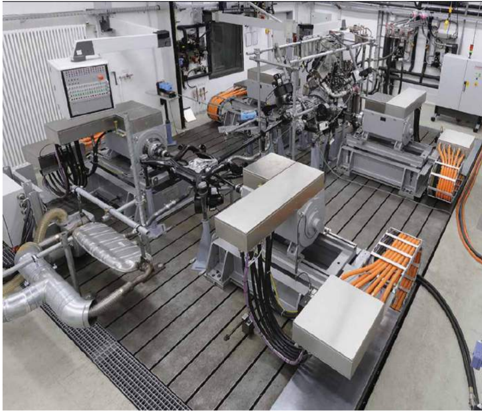
Fig. 1: Typical test bench configuration for a complete vehicle powertrain, [1].
