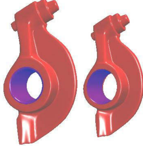
Fig. 6. Constrained scaling of a rocker arm: before scaling (left), after scaling (right) with S_x = 0.8 , S_y = 0.85 and S_z = 0.9 .
