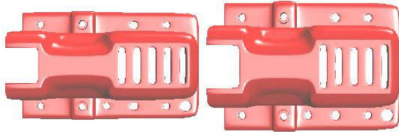
Fig. 7. Constrained scaling of a ventilation control component with three features: before scaling (left), after scaling (right) with S_x = 1.0 , S_y = 1.2 and S_z = 1.0 .
