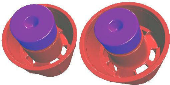
Fig. 9. Constrained scaling of a marker cap: before scaling (left), after scaling (right) with S_x = 1.2 , S_y = 1.2 and S_z = 1.0 .
