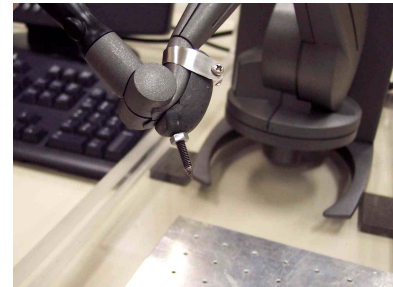
(b) Close-up of the probe (dm=0.5 mm)
