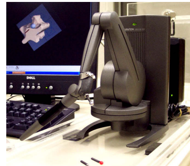
(a) PHANToM ® with a probe (dm=6.5 mm)
