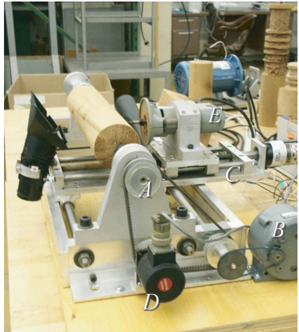
Fig. 4. Our prototype milling lathe. Labeled in the lathe photograph are the spindle (A), a DC motor (B) driving the tool carriage (C), the encoder (D), and the router (E).
